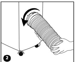
**2.** Twist the Exhaust Hose Connector over the discharge opening on the back of the unit and extend the Exhaust Hose. (Keep the exhaust hose as short and straight as possible)
