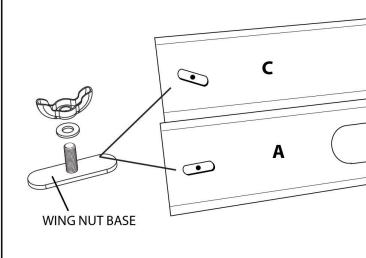
3. Place the Panel B over the Wing Nut Base on Panel C.
