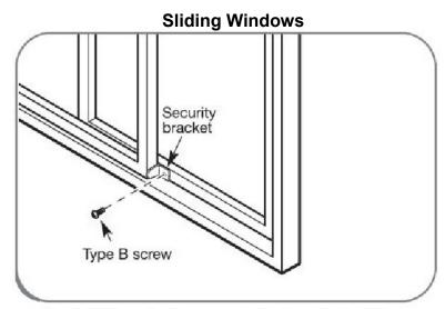
Install the window security bracket with a type B screw as shown.
