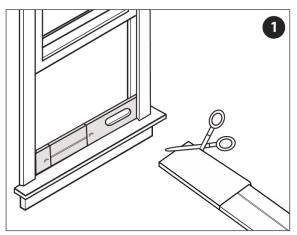
**1.** Open the window or door to adjust the length of the Window Kit Panels to fit the opening. If necessary, mark the kit and cut one end down to properly fit the opening.
