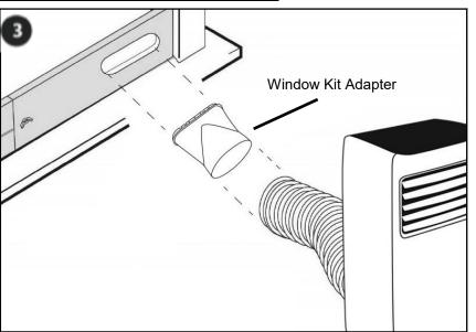
Keep the exhaust hose as short and straight as possible for maximum efficiency.
