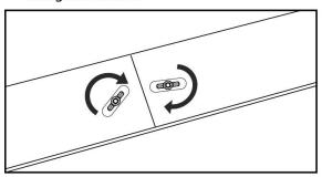
6. To complete the assembly, tighten the Wing Nuts installed earlier.
