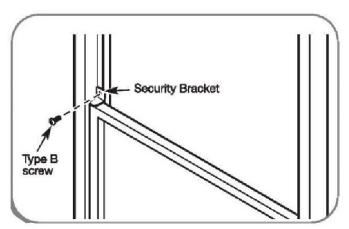
Install the security bracket with a type B screw as shown if you need.
