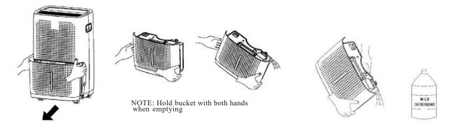
NOTES: When the bucket is full or removed from the dehumidifier, the compressor will turn off, but the fan may continue to run for a few minutes. This is completely normal. The dehumidifier will not be removing moisture from the air at this time. When removing moisture from the air, the dehumidifier will exhaust warm air from the top exhaust vent. Do not place a full bucket on the floor because the bottom of the bucket is uneven.
